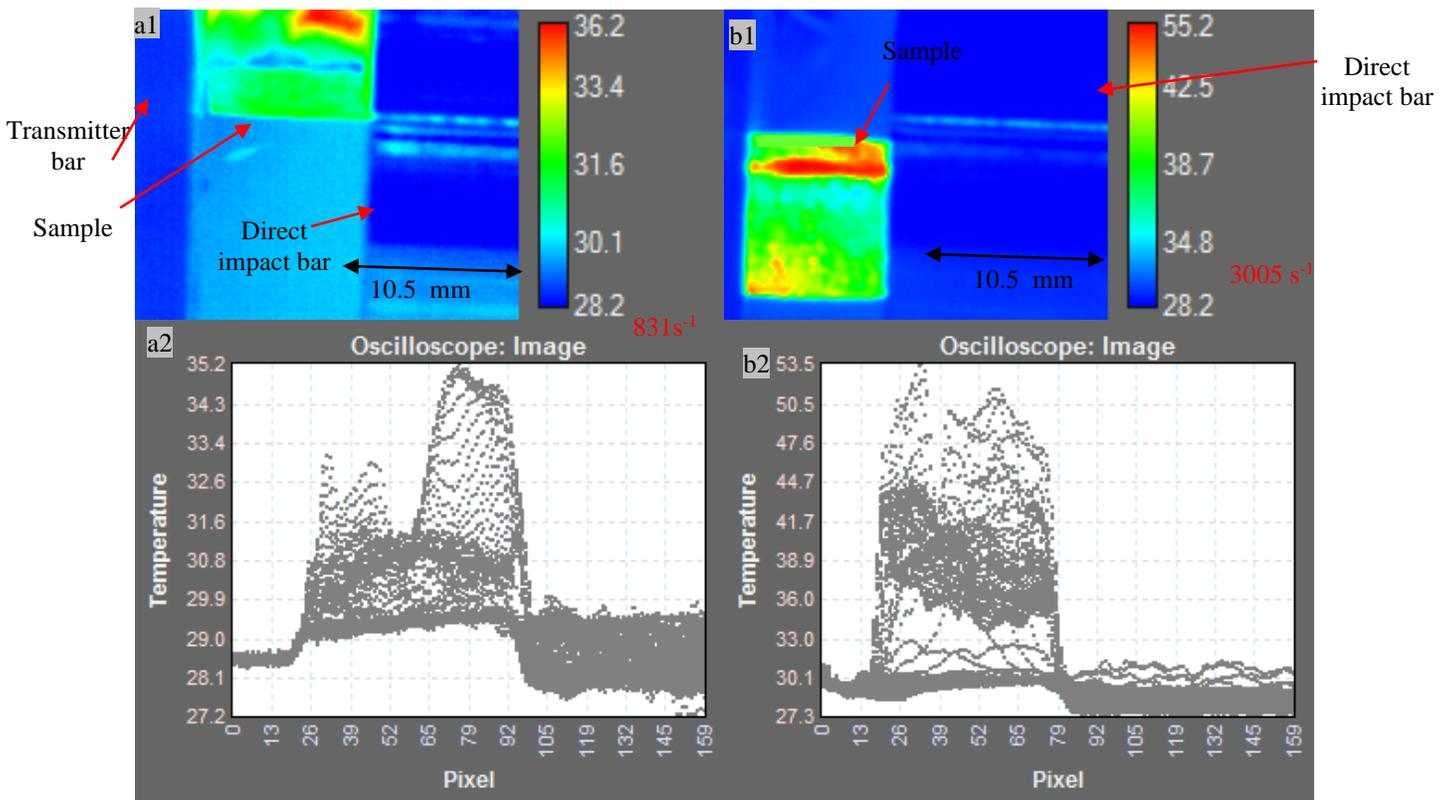
Figure 6. Effect of strain rates on temperature rise of specimen impacted at a)  $831 \text{ s}^{-1}$ , b)  $3005 \text{ s}^{-1}$ , a2 and b2 are the respective live profiles showing multiple nucleation site of temperature
