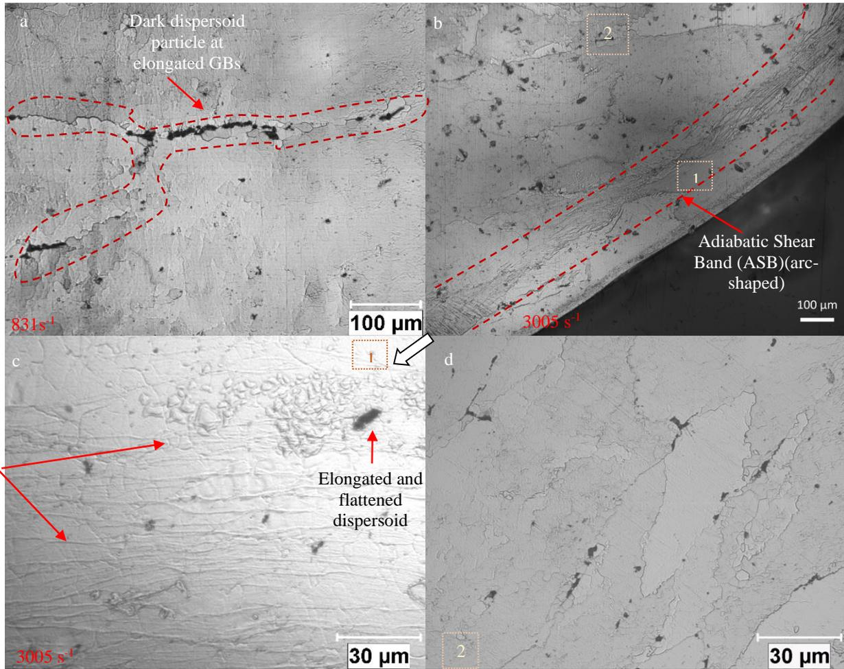
Figure 3: Microstructure after deformation showing aligned dispersoid particles at GBs at  $831 \text{ s}^{-1}$ , b) ASB zone with refined grains at  $3005 \text{ s}^{-1}$  c) dispersoids dynamic recrystallized grains within ASB region and d) deformed structure at ASB surroundings at  $3005 \text{ s}^{-1}$
