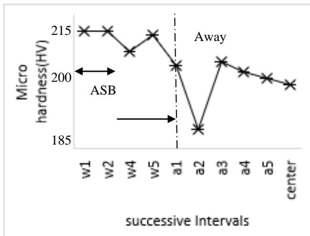
Figure 4. Microhardness variation within(w) ASB and away(a) from ASB region (w1) to center of matrix
