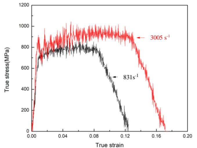
Figure 5. True stress-strain behavior of specimen impacted at  $831 \text{ s}^{-1}$  and  $3005 \text{ s}^{-1}$  strain rates
