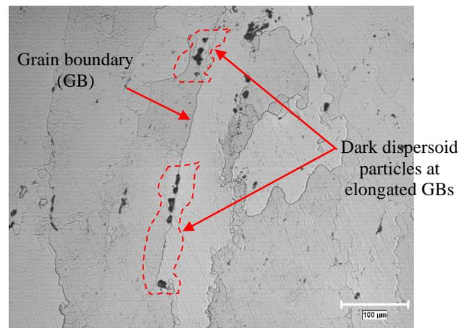
Fig. 2. Microstructure of un-impacted specimen showing elongated grains, globular shaped dispersoid particles at grain boundaries and sub grains
